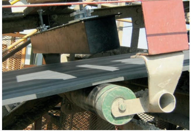
Ultrasonic sensor array complete with calming idler
